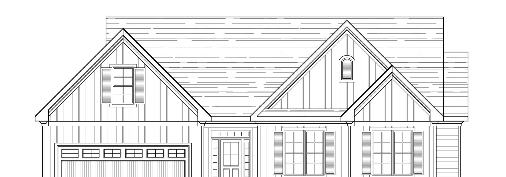
PROPOSED FRONT ELEVATION SCALE: 1/4"=1'-0"
